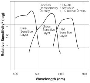
\* Sensitivity equals the reciprocal of the exposure  $(J/cm^2)$  required to produce a specified density.
